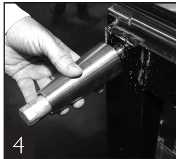
4 Thread leg into cabinet bottom frame rail.
