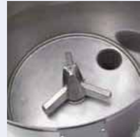
Residual water drain
