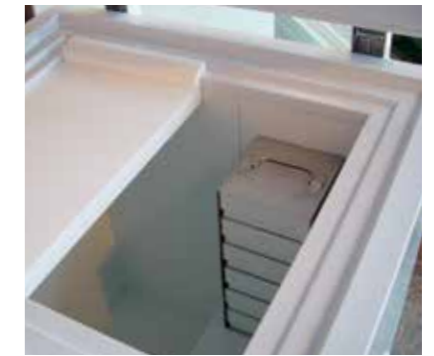
Inner lids (left hand side) which are mandatory for optimized function
